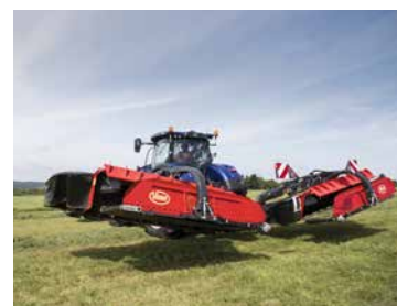
Ample clearance during headland lift. When belts are raised, they will automatically stop.
