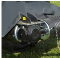
540/1000rpm turnable gearbox as standard.
