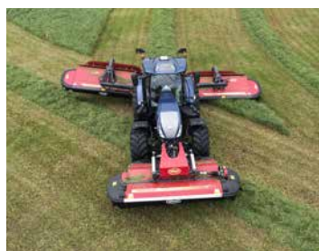
When using one belt only, speed is reduced to avoid crop being placed too far across the middle.
