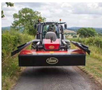
Hydraulic folding of FlexProtect guards (optional).
