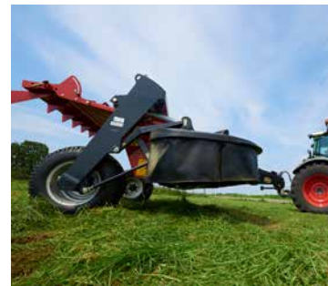
A lifting height of 500mm, ensures excellent ground clearance for transport and during headland turning.
