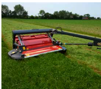
Fixed mainframe and reduced number of moving parts – less maintenance and wear.
