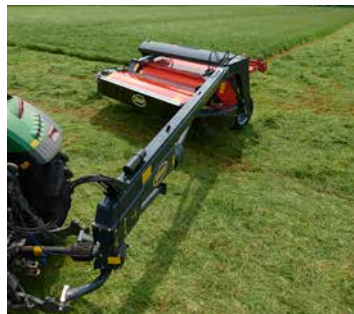
The swivel hitch headstock with reversible gearbox provides optimal manoeuvring ability.
