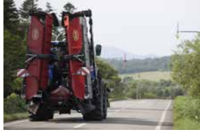
For transport, BX belts are positioned well within the cutting units.
