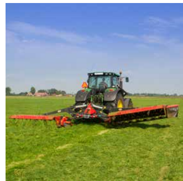
Each mowing unit can be lifted individually, convenient when mowing awkward shaped fields.
