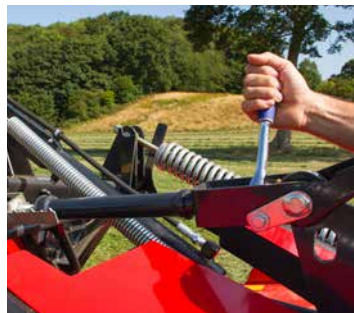
Stubble height adjustment is conveniently integrated directly into the suspension linkage. There is no need to tilt the A-frame of the tractor.
