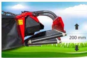
Vicon BX can deliver the crop at different working height.
